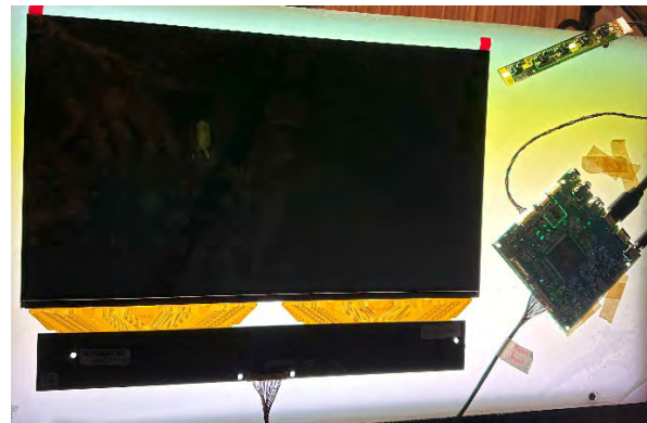
Opaque 13.3in LCD with driver & control boards
