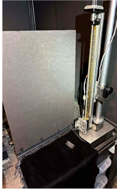
FUYU slit cable connector vulnerability. FUYU with attached light blocking with slit lowered to start height.
