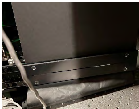
FUYU stage slit & H1 light blocking method.
