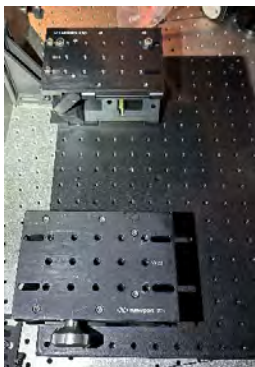
OPPH labjack support arrangement & right front labjack top screw arrangement & breadboard attachment closeup.
