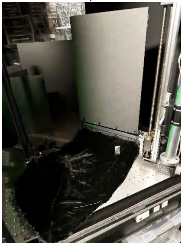
FUYU stage slit & H1 light blocking method.
