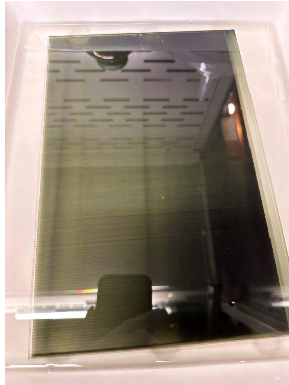
Hypericum H1 slit master in 90% ethanol to 10% water bath.
