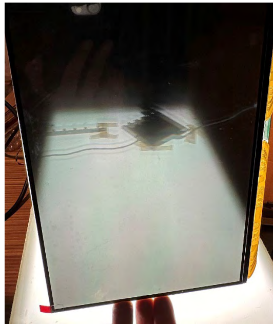
Diffraction transmissive ghosting in LCD
