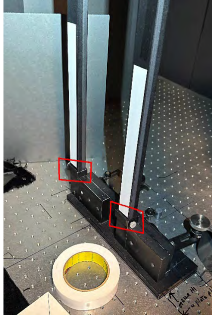
Doublestick tape applied to H1PH legs and plate stops (outlined in red) in better position.
