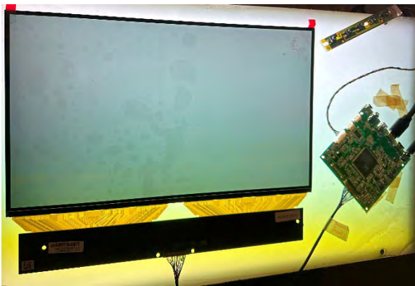
Clear 13.3in LCD with driver & control boards
