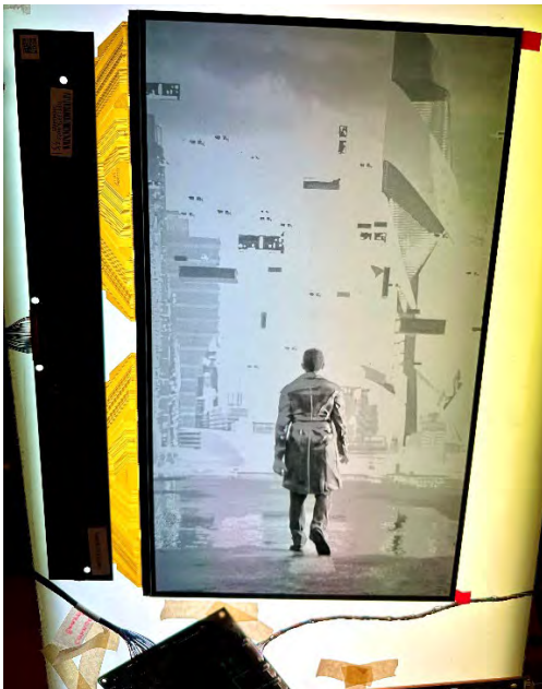
4K 13.3" transmissive monochrome LCD
