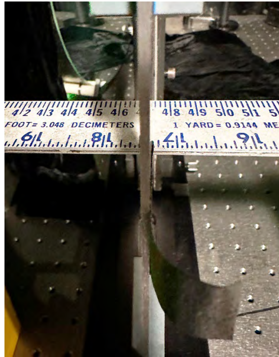
Setting & checking OB H1 plane to projection screen plane distance.
