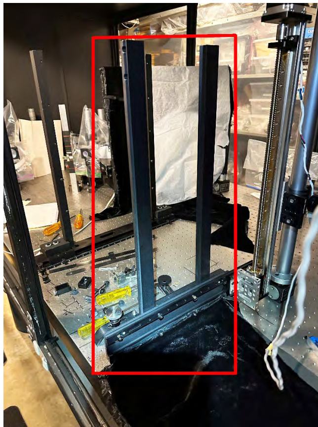
Customized DO5151 H1 plateholder with slit plate positioned at bottom
