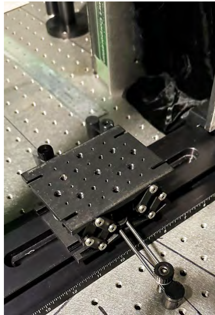
Thorlabs L200 labjack for vertical adjustment of projection screen.
