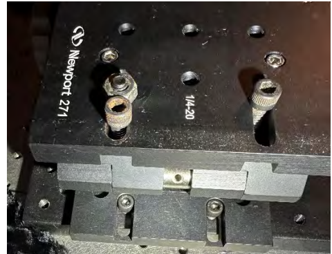
OPPH labjack support arrangement & right front labjack top screw arrangement & breadboard attachment closeup.
